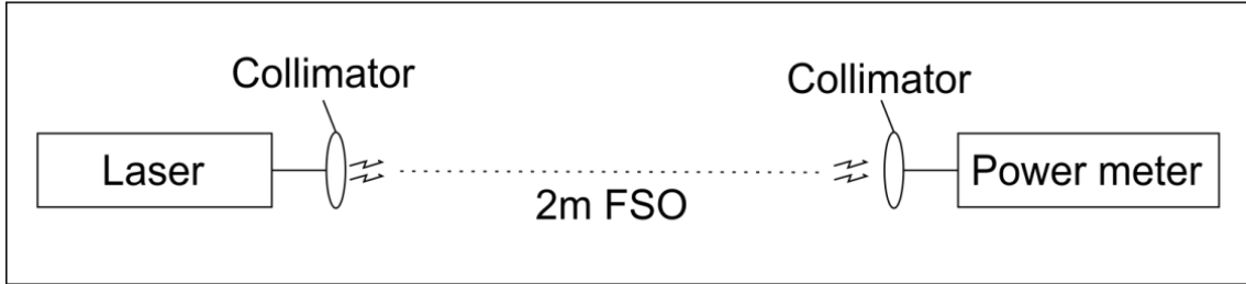
Figure 15 – Schematic block for continuous wave transmission
